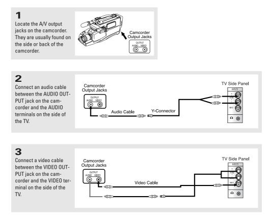
The audio-video cables shown here are usually included with a Camcorder. (If not, check your local electronics store.) If your camcorder is stereo, you need to connect a set of two cables.
